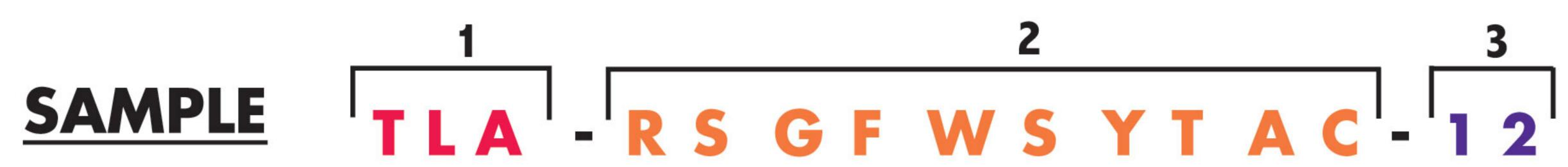
The sample shown, Part No. **TLA-RSGFWSYTAC-12**, is a 24V DC tower light assembly that has one red solid light, one green flashing light, one white solid light, and one yellow turning light (stacked from bottom to top). It also has a continuous tone alarm with a 12" (304 mm) pipe extension.
