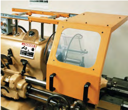
Shield slid into position. Machine is ready for machining workpiece.
