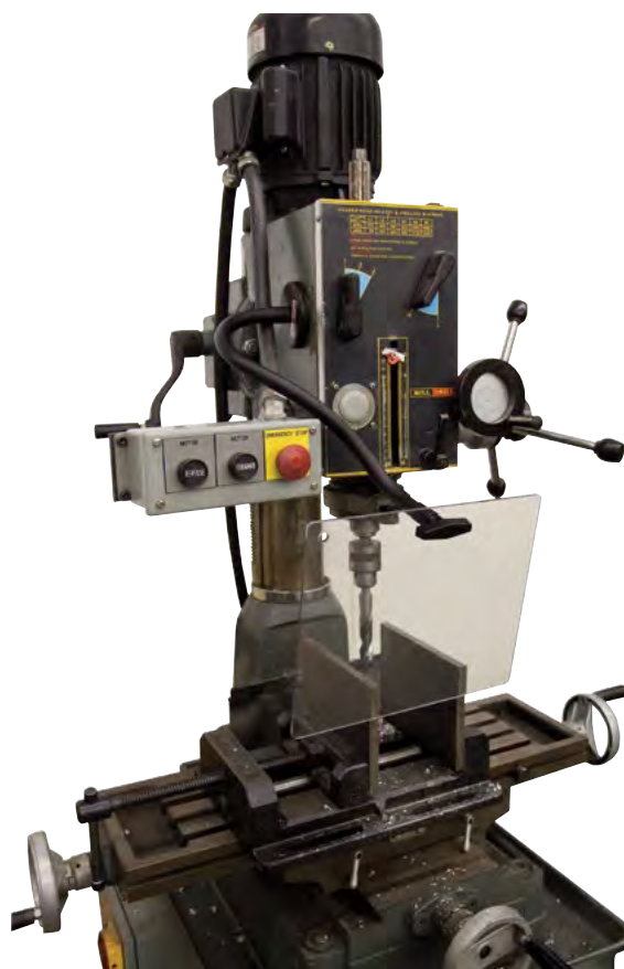
Flexible spring-steel arm shield on milling machine.
