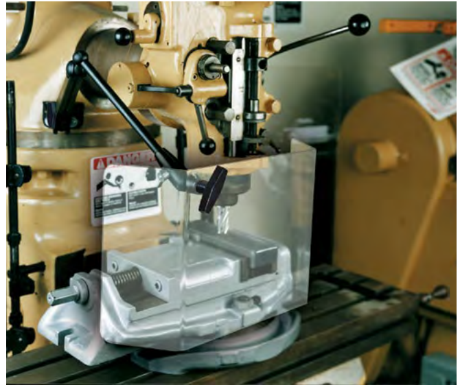
Universal ball & socket shield on a milling machine.
