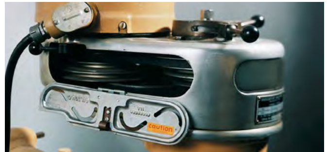
Cover open on model J Bridgeport milling machine.
