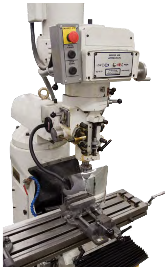
Flexible spring-steel arm shield on milling machine.
