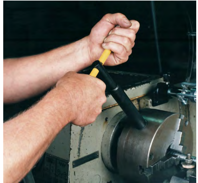
Adjusting the chuck using a spring-loaded chuck wrench.
