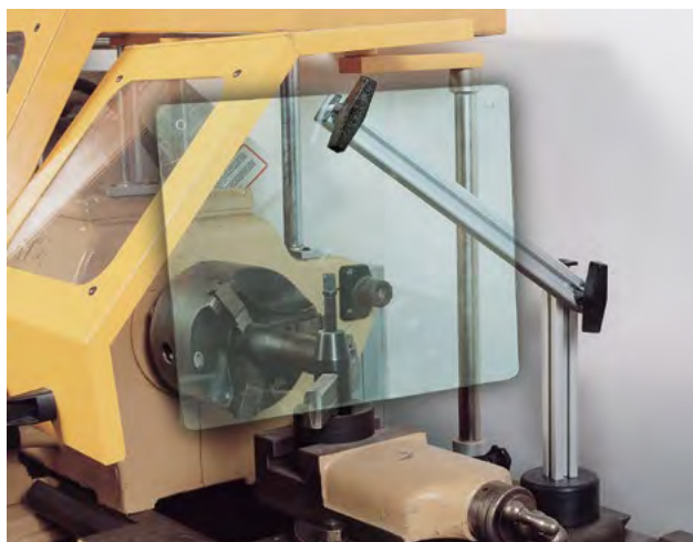
Magnetic-base flat shield shown on a lathe
