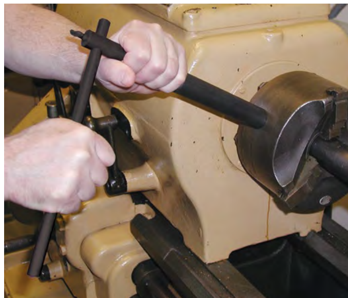
Adjusting the chuck using a long-handed spring-loaded chuck wrench.
