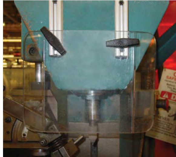
Adjustable slide shield on front column of machine.
