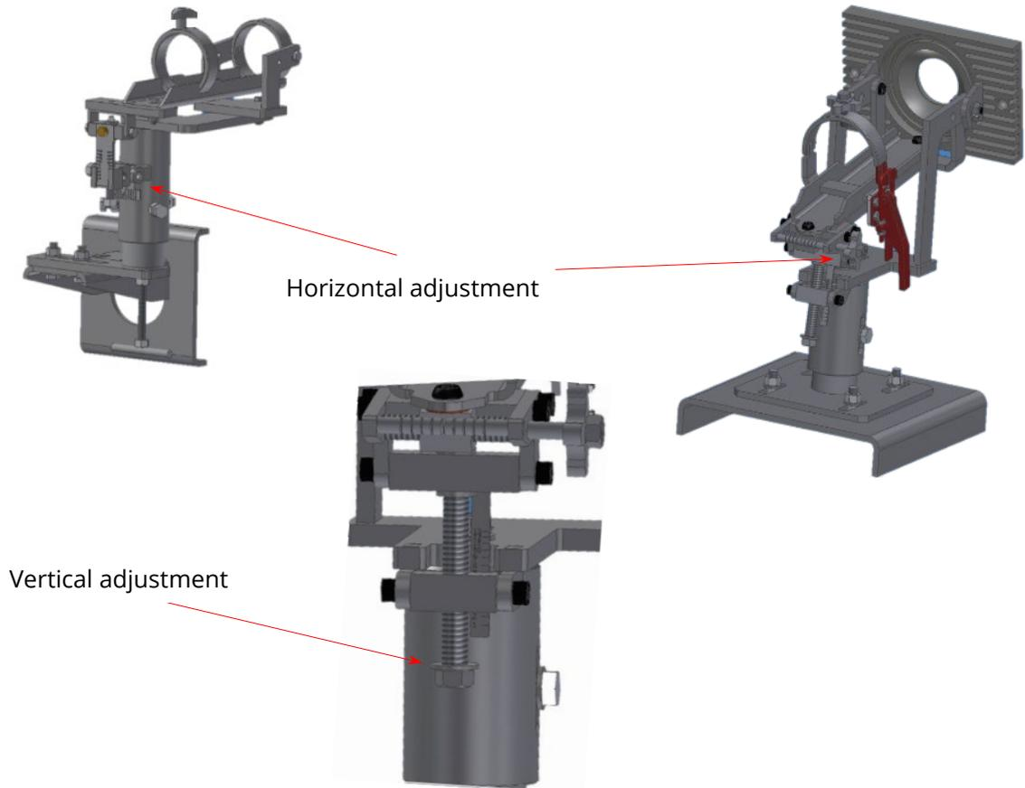
Figure 2. FlexFire® burner Adjustment Mechanism
