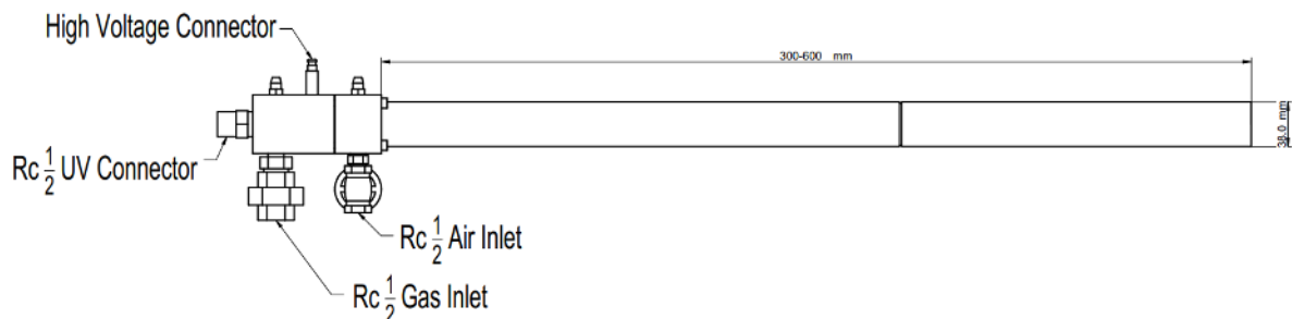
Figure 1: PBA90 Series air burner
