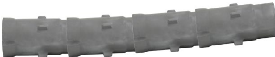
Figure 2: Self-recuperative burner inner tube
