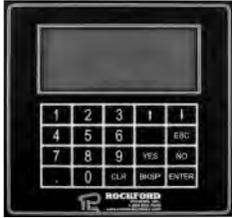
The keypad/display is used to enter setup information and to monitor machine operation. The keypad/display can be furnished in a remote enclosure up to a maximum of 150' from the control module. All programming is accessed by a keyed selector switch on the keypad/display unit.
