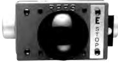
The red emergency-stop button is used to stop the machine anywhere in its cycle. When the operator depresses the button, it should stop the hazardous motion of the machine immediately by shutting off the hydraulic drive pump motor. This palm button assembly includes a double hub mounting box. It can be located between the two run palm buttons as part of the operator's control station. This button has a mechanical latch that must be reset after depressing the button.
