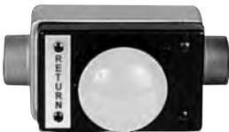
The yellow return/inch-up button is used to stop the machine when it is in the automatic mode of operation. When the operator depresses the button, almost anywhere in the stroke of the machine, it will return the ram to the up position. This palm button assembly includes a double hub mounting box. It can be located between the two run palm buttons, along with the red emergency-stop button, as part of the operator's control station.
