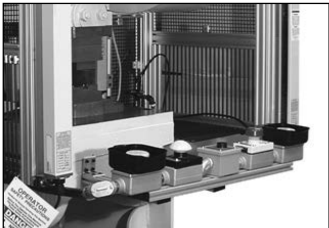
Touchdown!™ palm button assembly on a mechanical power press.
