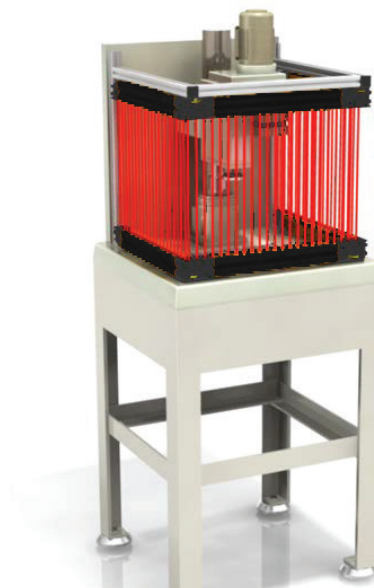
Figure 45. Cascaded light screens guarding a u-shaped cell
