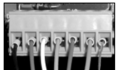
Photo 3.20—Terminal Strip P1 Wiring Connection on the Crankshaft Angle Display
