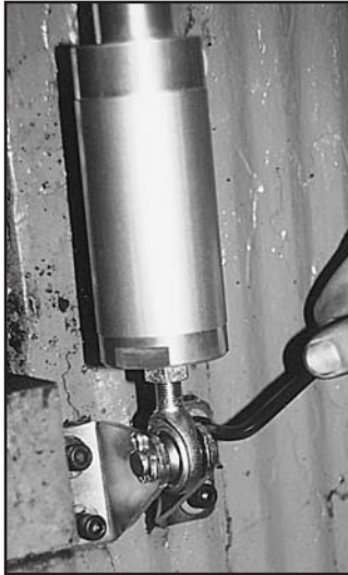
Figure 3.5 Standard Pull Cylinder with Clevis Mount
