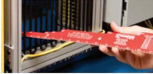
The critical role of measuring barrier openings falls on a simple but often misunderstood tool: the Guard Opening Scale. Also known as “gotcha sticks,” Guard Opening Scales mimic the human hand and forearm. **Over the past 70 years they’ve proven to be the most accurate means of ensuring any opening in a barrier guard will not allow a hazardous zone to be accessed.**
